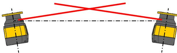
Figure 17. Scanners mounted at different scanning angles
