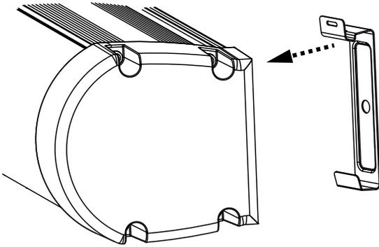
Figure 1. Attaching the snap brackets (step 6)
