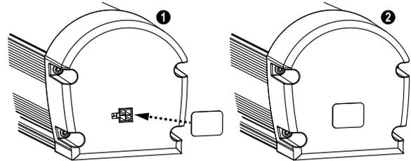
Figure 2. Installing the cascade cover (step 9)
