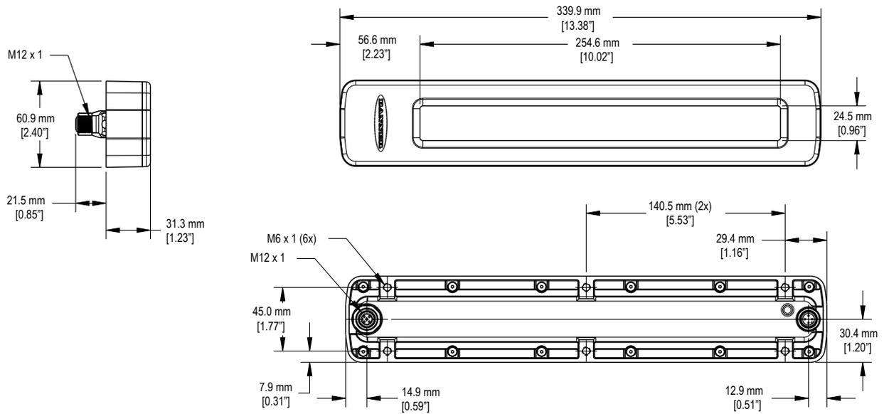
Figure 2. WLC60 (340 mm) Base Mount Rear Exit Models
