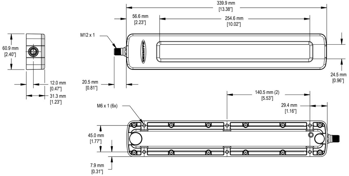
Figure 1. WLC60 (340 mm) Base Mount Side Exit Models
