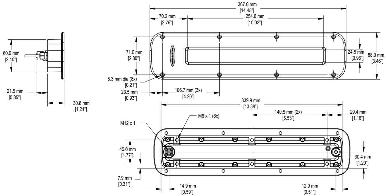
Figure 3. WLC60 (340 mm) Flush Mount Models
