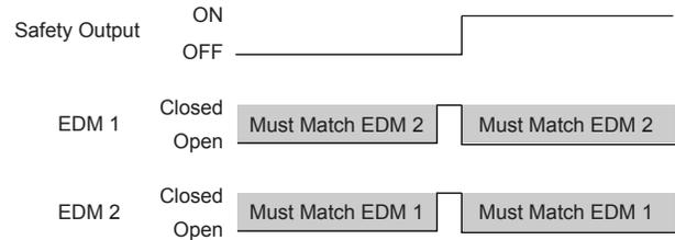
Figure 38. Timing logic: Two-channel EDM status, with respect to Safety Output
